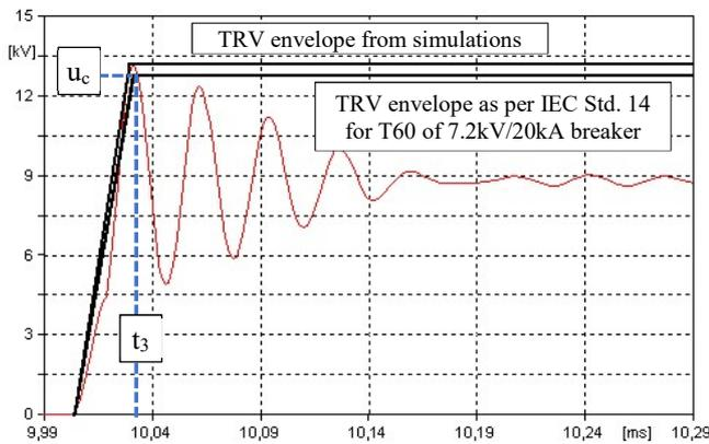
Fig. 14. Transient Recovery Voltage simulated for synthetic testing **with voltage injection**; with two two-parameter envelopes: for the TRV simulated, for the TRV according to IEC Std. 62271-100 (i.e. with  $u_c = 13.2$  kV, and  $t_3 = 22 \mu\text{s}$  as per Table I for T60)
