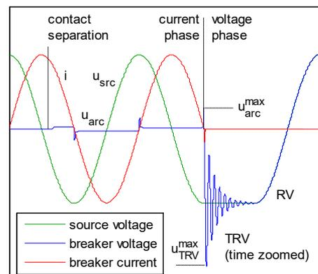
Fig. 1. Switching process of AC current with indicated high current phase for a breaker in closed position before current interruption, high voltage phase for a breaker in open position after interruption, and interaction phase in between the high current and high voltage phases [9]
