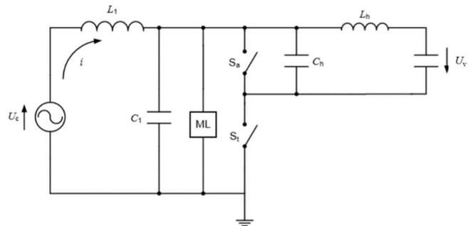
Fig. 7. Typical voltage injection circuit with voltage circuit parallel to auxiliary circuit-breaker [14]:  $U_c$ ,  $U_v$  – voltages of current and voltage circuits,  $L_1$ ,  $L_h$  – inductances of current and voltage circuit,  $ML$  – multi-loop re-ignition circuit,  $S_a$ ,  $S_t$  – auxiliary and test circuit-breaker,  $C_1$ ,  $C_h$  – Capacitances forming transient recovery voltages
