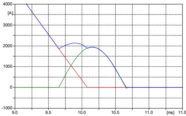
Fig. 9. Current waveforms simulated for synthetic testing **with parallel current injection**; red color – current at the current circuit (through the auxiliary switch), green color – current at the voltage circuit, blue color – current at the test circuit breaker
