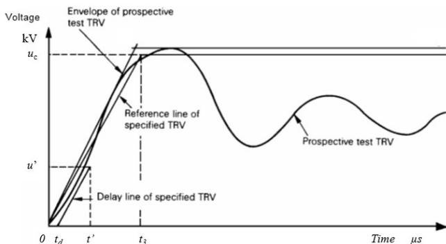
Fig. 3. Example of transient recovery voltage along with its envelope with the standardized parameters marked to meet the type test requirements [17]
