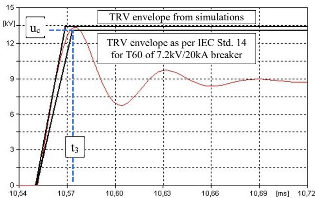
Fig. 10. Transient Recovery Voltage simulated for synthetic testing **with parallel current injection**; with two two-parameter envelopes: for the TRV simulated, for the TRV according to IEC Std. 62271-100 (i.e. with  $u_c = 13.2$  kV, and  $t_3 = 22 \mu\text{s}$  as per Table I for T60)
