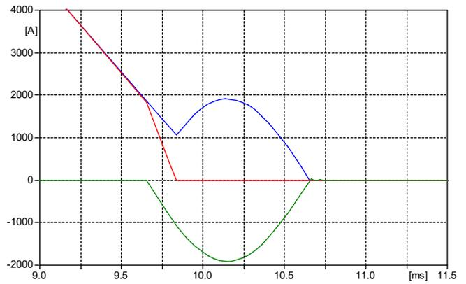
Fig. 11. Current waveforms simulated for synthetic testing **with series current injection**; red color – current at the current circuit (through the auxiliary switch), green color – current at the voltage circuit, blue color – current at the test circuit breaker
