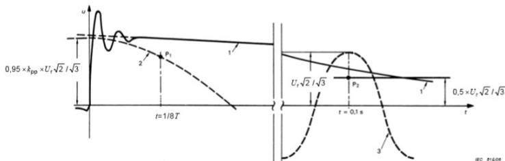
Fig. 4. Prospective transient recovery voltage [14]: 1 – recovery voltage across circuit-breaker during a synthetic test, 2 – power frequency recovery voltage of first extinguishing pole in the equivalent direct test, 3 – power frequency recovery voltage after interruption of all currents
