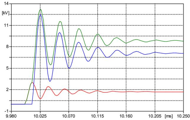
Fig. 13. Voltage waveforms simulated for synthetic testing **with voltage injection**; red color – voltage waveform from the current circuit, green color – voltage waveform from the voltage circuit, blue color – TRV at the test circuit breaker (a sum of the two latter voltage waveforms)
