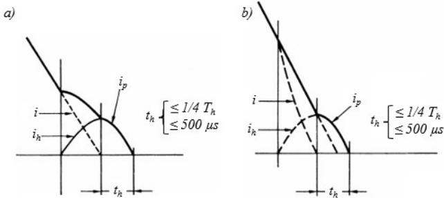
Fig. 6. Injection timing for parallel (a) and series (b) current injection [14]:  $i$  – current from current circuit,  $i_h$  – injected current from voltage circuit,  $i_p$  – current in tested circuit-breaker,  $t_h$  – time during which the arc is fed only by the injected current
