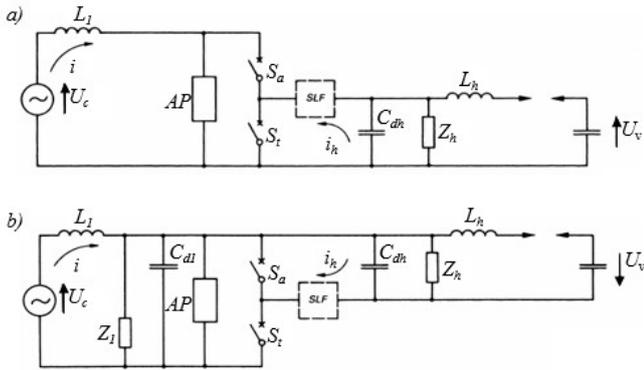
Fig. 5. Typical current injection circuits with voltage circuit parallel to test (a) and auxiliary (b) circuit-breaker [14]:  $U_c$ ,  $U_v$  – voltages of current and voltage circuits,  $L_1$ ,  $L_h$  – inductances of current and voltage circuits,  $AP$  – arc prolonging circuit,  $S_a$ ,  $S_t$  – auxiliary and test circuit-breakers,  $C_{dh}$ ,  $C_{db}$ ,  $Z_1$ ,  $Z_h$  – impedance forming transient recovery voltage
