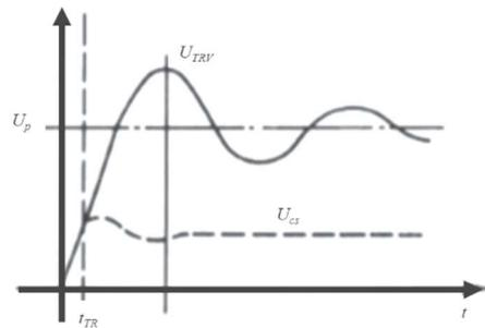
Fig. 8. Transient recovery voltages in voltage injection circuit:  $U_{cs}$  – transient recovery voltage from current circuit,  $U_p$  – power-frequency recovery voltage,  $U_{TRV}$  – transient recovery voltage on test circuit breaker,  $t_{TR}$  – time instance of switching of the voltage circuit
