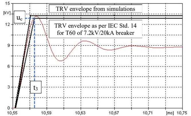
Fig. 12. Transient Recovery Voltage simulated for synthetic testing **with series current injection**; with two two-parameter envelopes: for the TRV simulated, for the TRV according to IEC Std. 62271-100 (i.e. with  $u_c = 13.2$  kV, and  $t_3 = 22 \mu\text{s}$  as per Table I for T60)
