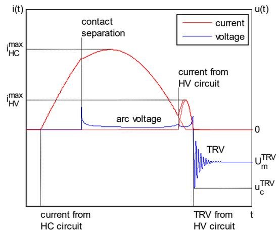
Fig. 2. Current and voltage waveshapes in Parallel Current Injection Synthetic Test Circuit [9]
